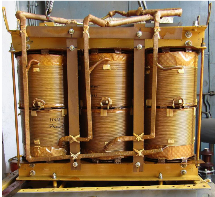
PHOTOGRAPH SHOWING TRANSFORMER AFTER S.C. TEST
